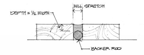
It's important to realize that caulking joints need to have the proper depth-to-width ratio or they will fail. Caulking should never be used as the only barrier to keep moisture out. Caulking joints also require maintenance every 3-5 years.
